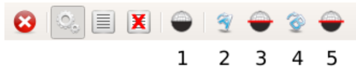
Figure 30: Edit modes reachable via the upper toolbar. 1. Toggle clipping for both representations. 2. Move first representation. 3. Edit clipping height for first representation. 4. Move second representation. 5. Edit clipping height for second representation.
