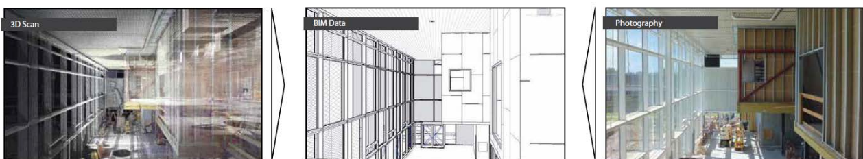
Fig.: 1 3D Scan, BIM, Images – The types of data under investigation in the DURAARK project
