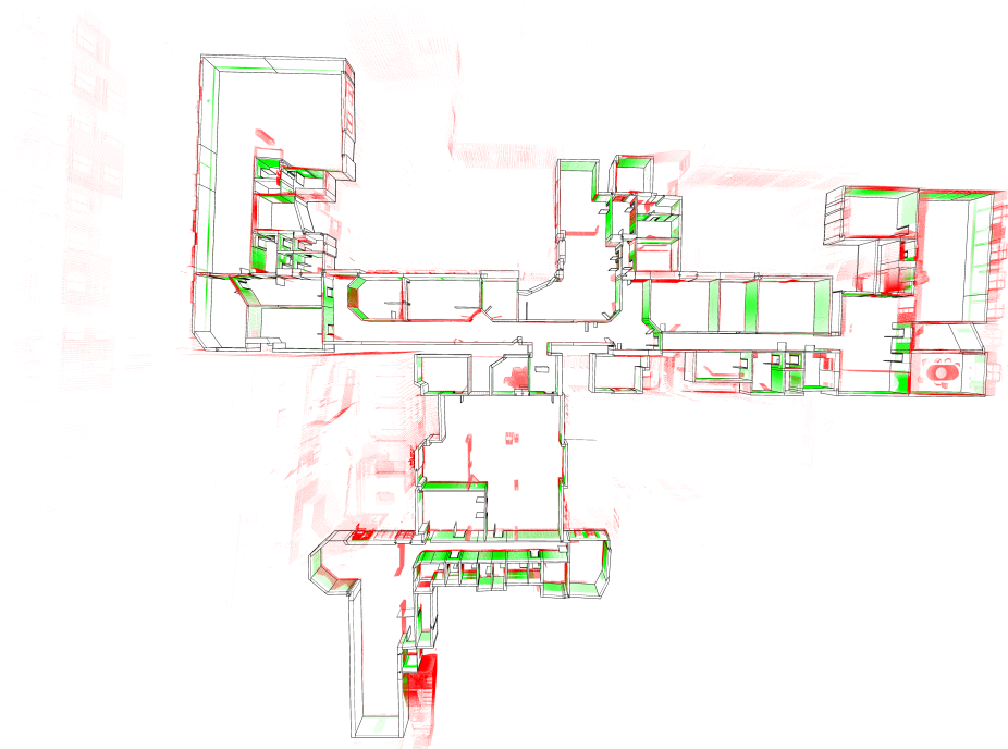
Figure 53: Difference Detection of automated reconstructed BIM model and Point Cloud easing the inspection of the model resulting from the registration component. Green depicts points considered associated with objects. Red depicts points considered not associated with objects.
