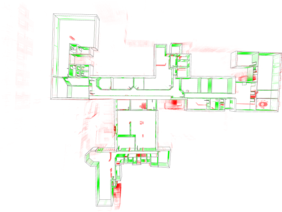
Figure 54: Difference Detection of corrected BIM model and Point Cloud. This gives salience to the inspection of the resulting model. Green depicts points considered associated with objects. Red depicts points considered not associated with objects.
