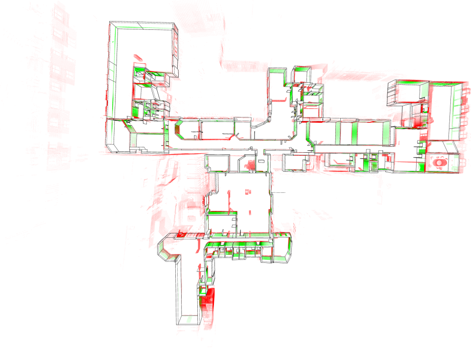
Figure 17: The difference between a BIM model and an E57 pointcloud. The architect realizes a large difference (red indicates large differences, green no or only small differences) and reconstructs a new BIM model using the IFC Reconstruction component.
