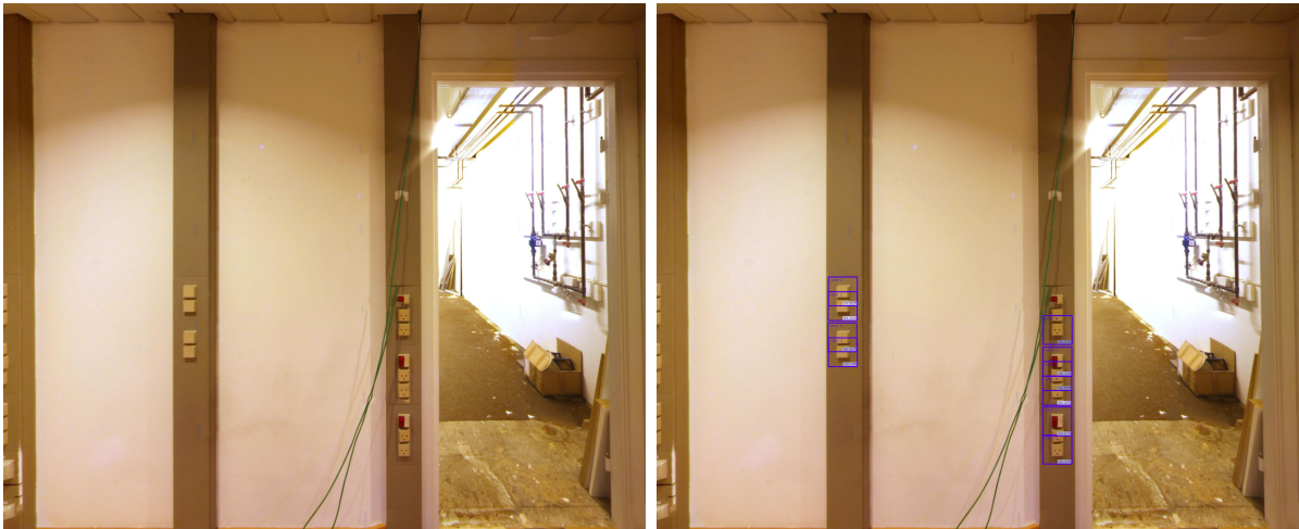
Figure 7: The ElecDetect module performs the detection of sockets and switches (right) on orthophotos generated by the OrthoGen module (left).
