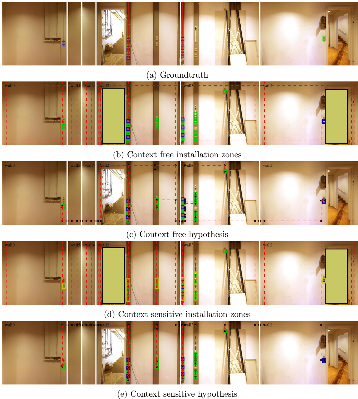
Figure 12: A groundtruth for nygade1001 has been manually acquired (a). A context free grammar (b) yields wrong results (c) in regions where groups of sockets and switches suggest an additional zone. A context sensitive grammar (d) that creates additional zones where groups are found (yellow rectangles) yields a correct result (e).
