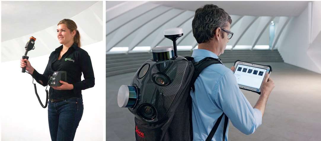
Figure 58: The ZEB1 Hand-held 3d sensor and the Leica Pegasus Backpack are commercial indoor 3d registration techniques, that are mobile and faster than 3d laserscanning.
